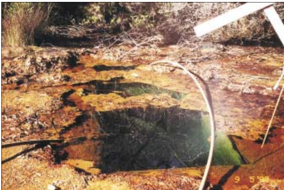
Plate 2. Acid drainage in open shaft at the Balfour copper mine
