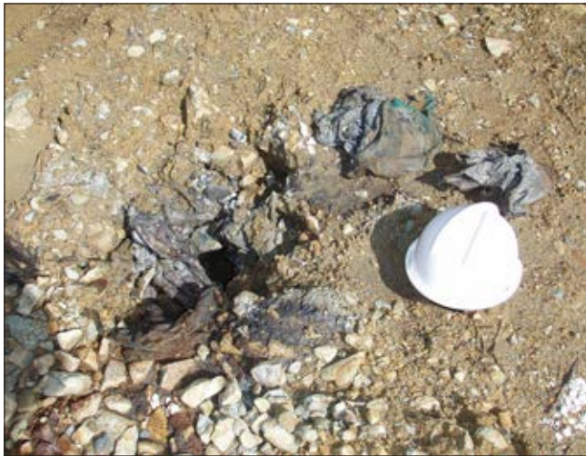
Open hole jammed with grease-soaked rags.
