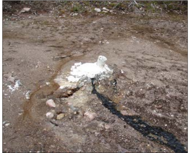
Three attempts to seal hole with eventual success at great cost. Note no solid secure collar.
